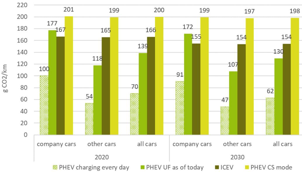
Figure 8.4: CO<sub>2</sub> tailpipe emissions per km for PHEV and ICE, 2020 and 2030. Source: own calculations.
