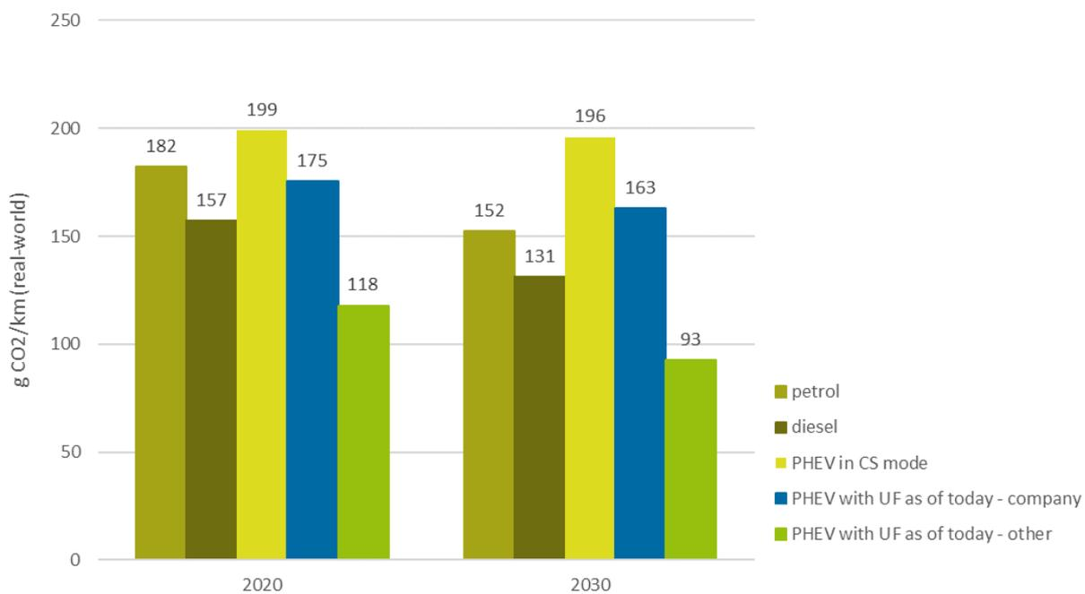
Figure 8.1: CO<sub>2</sub> emissions per km for PHEV and equivalent ICEV (weighted average)
