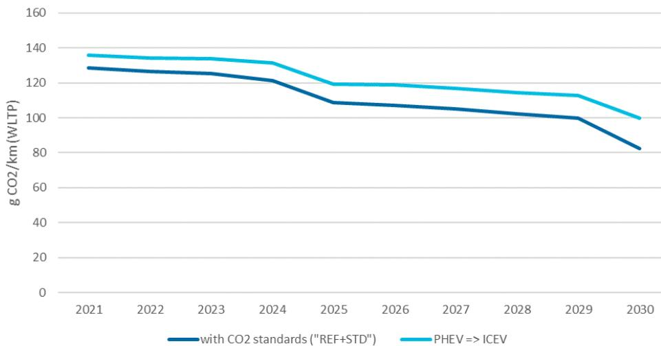
Figure 8.3: WLTP CO<sub>2</sub> emissions per km for new registrations in Germany. Source: own calculations.
