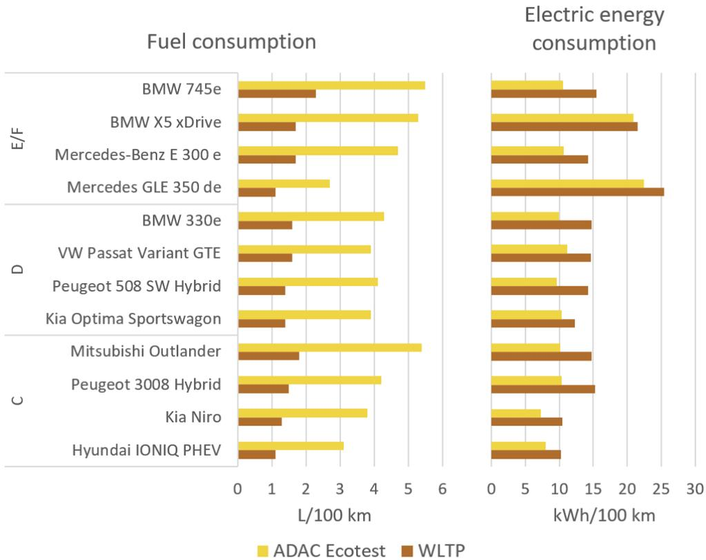
Figure 5.2: Comparison between WLTP and ADAC Ecotest fuel and electric energy consumption (combined values)
