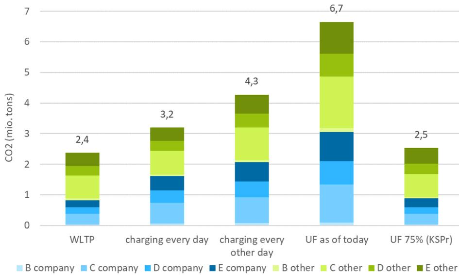
Figure 7.5: Total PHEV CO<sub>2</sub> emissions in Germany 2030 for different charging behaviours
