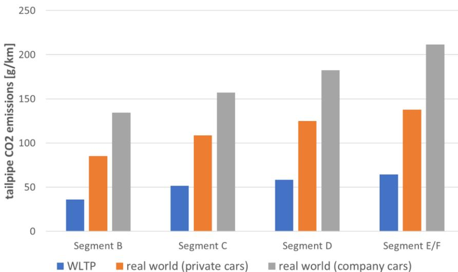
Figure 5.12: Tailpipe CO<sub>2</sub> emissions for defined vehicle segments, baseline 2020 (own calculations)
