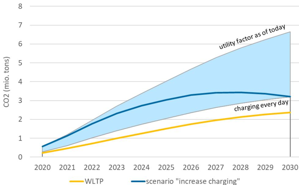
Annual tailpipe CO<sub>2</sub> emissions from PHEV in Germany in the timeframe 2020-2030 based on WLTP assumptions (yellow) and different real-world charging assumptions (blue).
