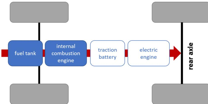
Figure 2.2: Exemplary topology of a serial hybrid powertrain
