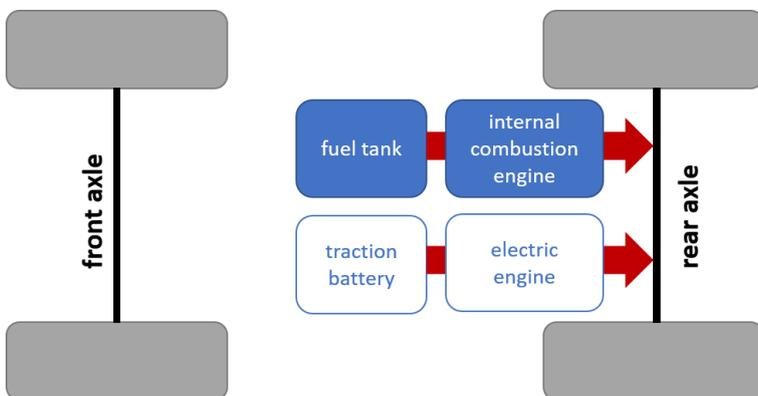
Figure 2.1: Exemplary topology of a parallel hybrid powertrain
