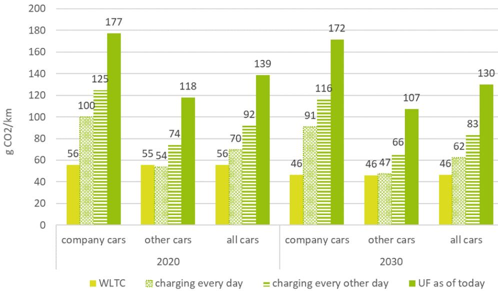
Figure 7.4: PHEV CO<sub>2</sub> tailpipe emissions per km depending on charging behaviour, 2020 and 2030
