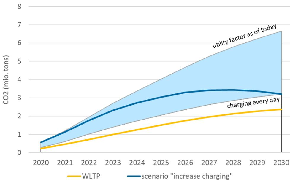
Figure 7.6: Total PHEV CO<sub>2</sub> emissions in Germany in the case of increased charging, 2020-2030
