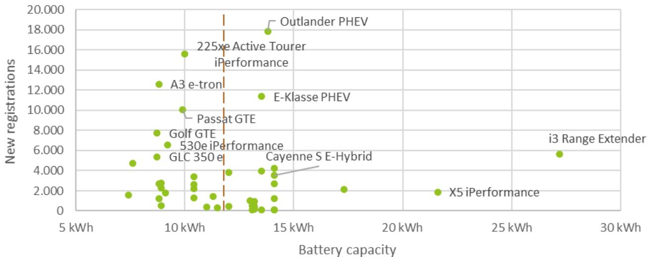
Figure 4.14: Number of PHEV new registrations by battery capacity from 01/2015 to 03/2020. The dashed red line shows the sales-weighted capacity average.
