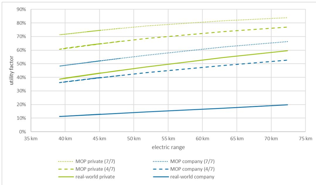
Figure 6.7: Utility factors applied in the scenario calculations; based on the mobility panel (MOP) for charging every day (dotted) and every other day (dashed) as well as based on empirical data from (Plötz et al. 2020).
