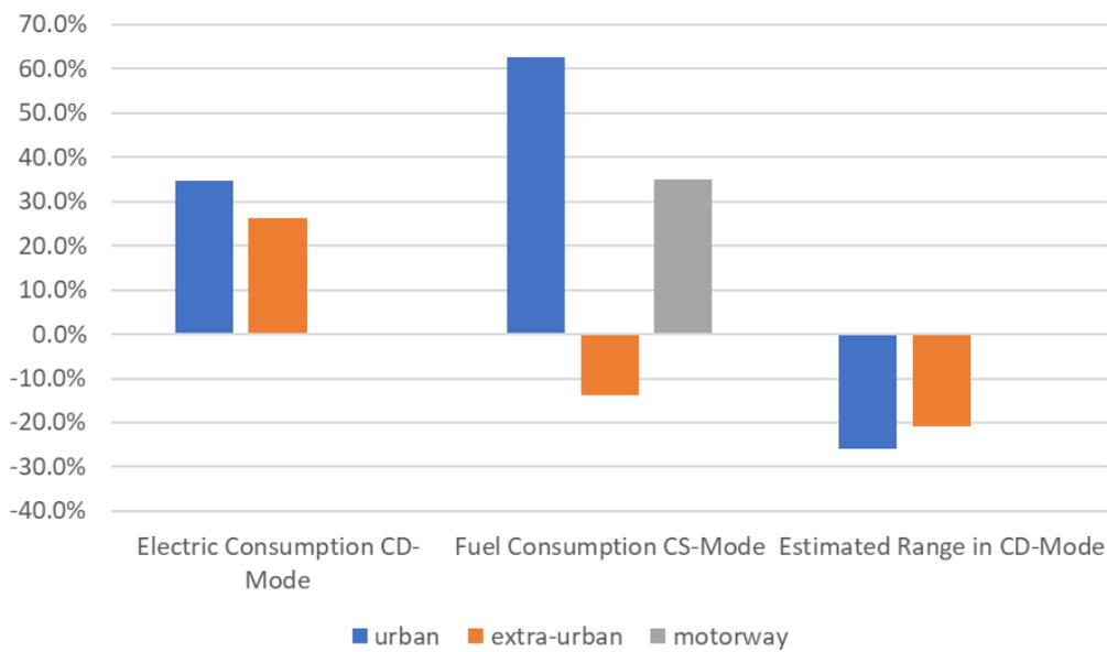
Figure 5.8: Discrepancy of electric consumption, fuel consumption and all-electric range for the example vehicle in HBEFA cycle simulation as compared to WLTP (own calculations)
