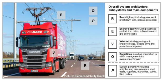
Figure 1: Overall system architecture and subsystems of the overhead contact line truck system (Image source: Siemens Mobility GmbH with additions by the author)
