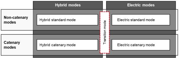
Figure 6: Interaction of the operating modes of an OH truck [after Schöpp et al. 2021b].
