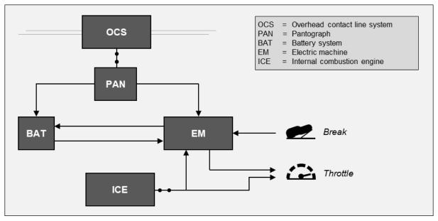
Figure 3: Simplified, schematic representation of the drive train of an OH truck [after Schöpp et al. 2022].
