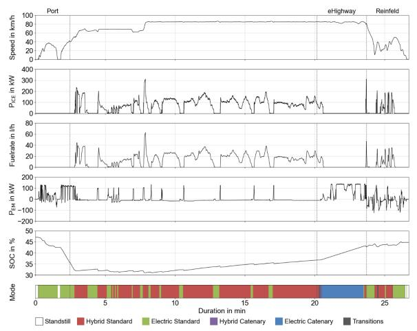
Figure 7: Curves of speed, mech. power of combustion engine and EM as well as SOC for an exemplary journey on the FESH test track
